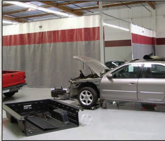
Create an Area to Work on Aluminum Vehicles to Eliminate Carbon Dust from Steel Vehicles Causing Rust on the Aluminum Finish.
