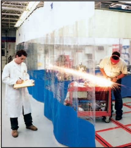
Control Grinding, Sanding & Buffing Contaminants or Separate Metal & Paint Shops
