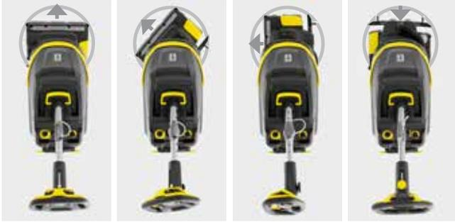
The roller brush head of the new BR 35/12 C Bp is an outstanding technical innovation: It can be horizontally rotated 200° in both directions around the steering axle. This means that every part of the full circle is covered, finally eliminating blind spots when cleaning. In the parking position, all pressure is taken off the brushes to prevent any damage.
