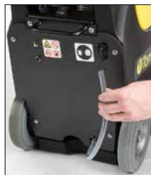
SITE TUBE The site tube at the rear of the machine allows the operator to easily see how much clean water/solution remains. The tube also allows for easy evacuation of any remaining unused water/solution.
